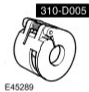
Fuel spring lock decoupling tool 310-005
